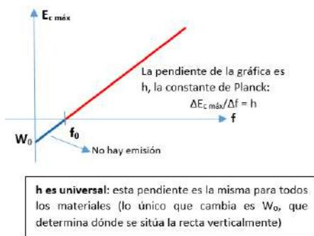
$hf = W_0 + E_{c \text{ máx}} \Rightarrow E_{c \text{ máx}} = hf - W_0$
